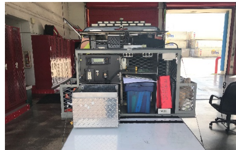
Figure 89: Rear Command Module - Slide out tray
