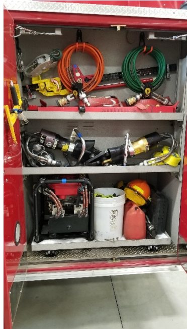
Figure 75: Engine 4 - Extrication Tools
