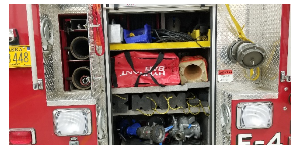
Figure 74: Engine 4 - Hard Suction Cabinet
