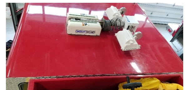
Figure 71: Engine 23 - Light Tower
