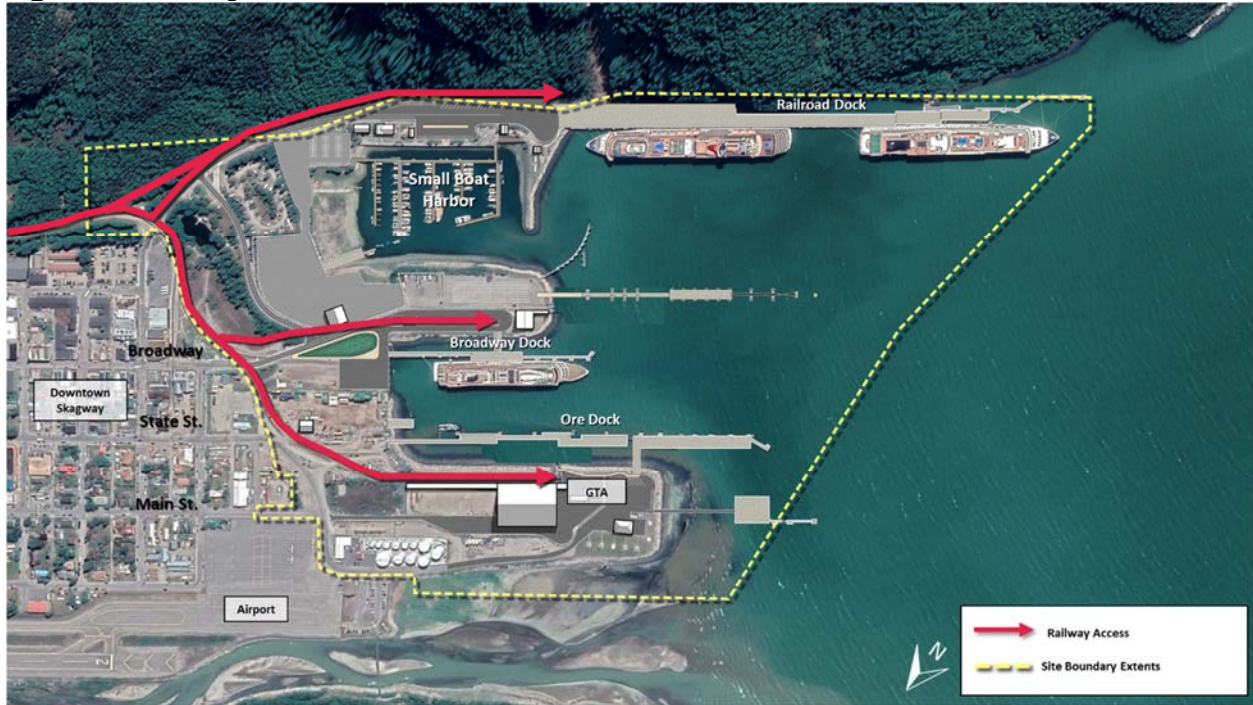
Figure 4: Railway Access Alternatives
